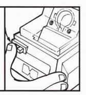
Do not open the clear cover until the machine is completely cooled down. After cooling, you can see an arrow pointing to the cool area inside the temperature indication chart. Then, you can crank the tilt plate down by turning away from you (clockwise) approximately 1/2 turn before you can open the clear cover. Make sure the knob snaps back into place after cranking back. The machine will not open unless the knob is locked
