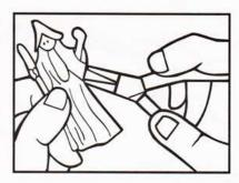
PLIERS CAN ALSO BE USED TO BREAK OFF FLASH AND RUNNERS FROM FIGURES.
