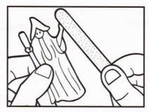
NA!L FILES (EMERY BOARDS) OR MEDIUM GRIT SANDPAPER CAN BE USED TO REMOVE FLASH OR RUNNERS FROM FIGURES.
