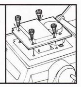
ARROW POINTING TOWARDS THE CRUCIBLE. THE BOTTOM HALF OF THE MOLD GOES INTO THE HOLDER WITH THE INSIDE (CAVITY AREA) FACING UP. BE SURE THAT THE "RUNNER" AREA OF THE MOLD HALF GOES UNDER
