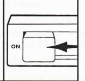
PULL THE KNOB ON THE RIGHT SIDE OF THE MACHINE OUT APPROXIMATELY 1/4 INCH AND TURN THE KNOB TOWARD YOU IN A SWIFT MOTION (COUNTER CLOCKWISE) APPROXIMATELY ONE HALF TURN.
