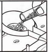
ONCE THE MOLD HALVES ARE IN CORRECTLY AND THE CRUCIBLE IS FULL WITH ONE VIAL OF METAL PELLETS, YOU MUST RETURN THE TILT PLATE COVER TO THE MACHINE AND TIGHTEN DOWN THE FOUR THUMB SCREWS COMPLETELY.
