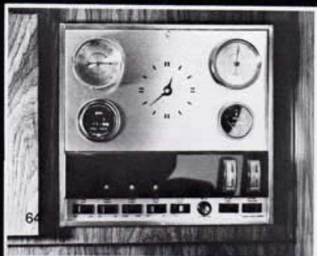
A COMPLETE WEATHER AND CENTRAL CONTROL PANEL ALLOWS YOU TO CONTROL THE AUXILIARY POWER OF THE COACH AS WELL AS CHECK ALL VITAL CAPACITIES AND INFORMATION.
