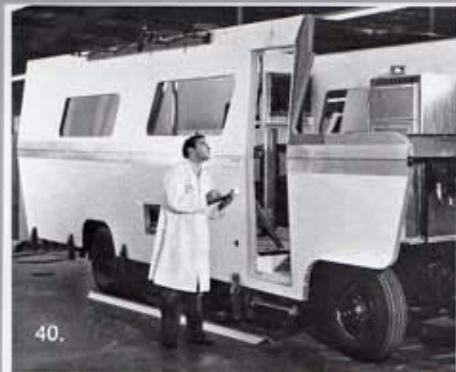
40. ONCE THE WALLS ARE IN PLACE THEY ARE INSPECTED AGAIN TO MAKE CERTAIN ALL SEAMS ARE EXACT IN THEIR FIT.
